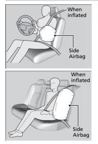
When the sensors detect a moderate-tosevere side impact, the control unit signals the side airbag on the impact side to immediately inflate.
