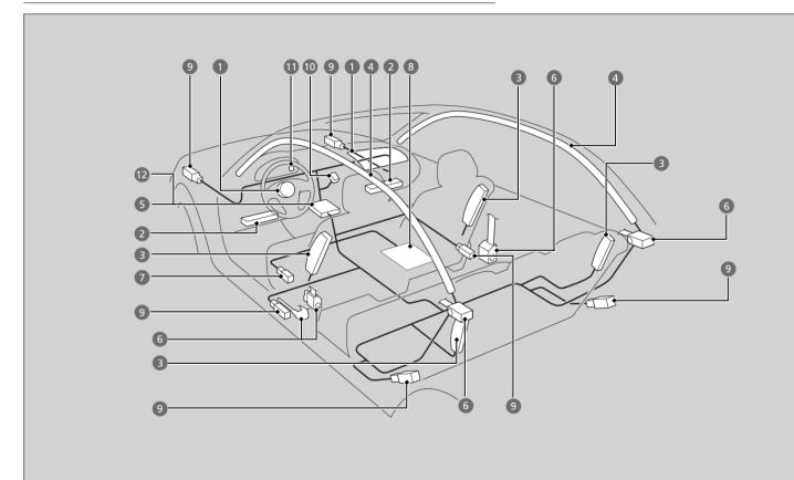
The front, driver's knee, front passenger's knee, side, and side curtain airbags are deployed according to the direction and severity of impact. Both side curtain airbags are deployed in a rollover. The airbag system includes:
