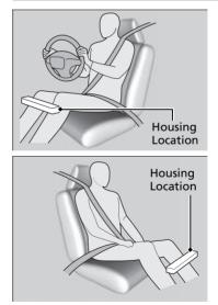
The knee airbag for the driver and the one for the front passenger are housed under the steering column and the glove box respectively.
