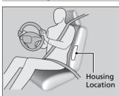
The side airbags are housed in the outside edge of the driver's and passenger's seatbacks and next to the outer rear seating positions.
