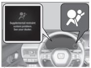
■ When the power mode is set to ON The indicator comes on for a few seconds, then goes off. This tells you the system is working properly. Supplemental Restraint System (SRS) Indicator
