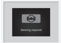
If the driver does not grip the steering wheel after the warning above has repeatedly appeared, a warning buzzer will sound and Traffic Jam Assist will be canceled
