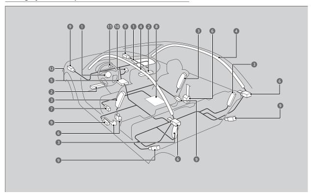
The front, front knee, side, and side curtain airbags are deployed according to the direction and severity of impact. Both side curtain airbags are deployed in a rollover. The airbag system includes:
