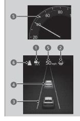
You can see the current state of Adaptive Cruise Control (ACC) with Low Speed Follow, Lane Keeping Assist System (LKAS) and Traffic Jam Assist.
