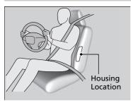
The side airbags are housed in the outside edge of the driver's and passenger's seat-backs and next to the outer rear seating positions.
