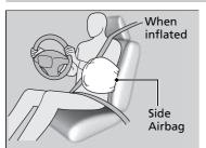
When the sensors detect a moderate-tosevere side impact, the control unit signals the side airbag on the impact side to immediately inflate.
