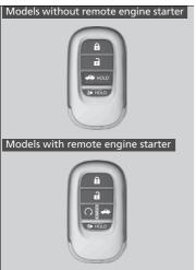
Use the keys to start and stop the engine, lock and unlock all the doors and the fuel fill door, and open the trunk.
