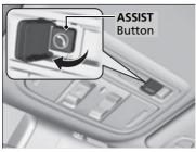
If you need to talk to the HondaLink® operator in a situation where no airbag has deployed, you can manually connect to them by pressing the **ASSIST** button with the power mode in ACCESSORY or ON.
