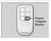
Press the power tailgate button for more than one second to operate when the power mode is in VEHICLE OFF.
