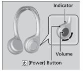
**To turn on the switch:** Press the **(**(power) button at the right earpiece. The indicator comes on.
