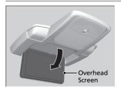
Pull down the screen to the first or second detent until it latches.
