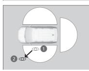
When you walk away from the vehicle with all doors and tailgate closed while carrying the keyless remote, the doors will automatically lock
