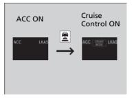
Press and hold the  $\boxed{\mathbb{Z}}$  (interval) button for one second. **Cruise Mode Selected** appears on the driver information interface for two seconds, and then the mode switches to Cruise.
