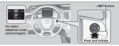
Take your foot off the pedal and press the **-/SET** button when you reach the desired speed. The moment you release the **-/SET** button, the set speed is fixed, and ACC begins.
