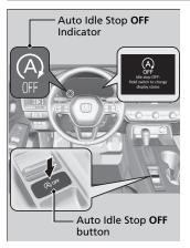
To turn the Auto Idle Stop system off, press this button. The Auto Idle Stop system stops.
