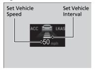
When ACC starts operating, the vehicle icon, distance bars and set speed appear on the driver information interface.
