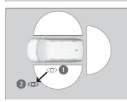
When you walk away from the vehicle with all doors and tailgate closed while carrying the keyless remote, the doors will automatically lock
