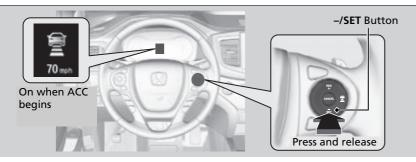
Take your foot off the pedal and press down the **-/SET** button when you reach the desired speed. The moment you release the **-/SET** button, the set speed is fixed, and ACC begins.
