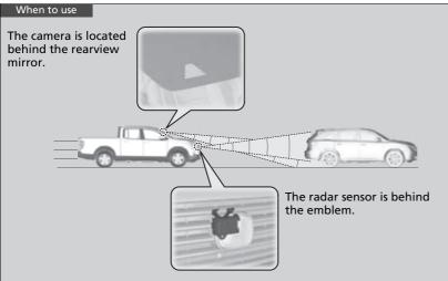
Vehicle speed for ACC: Desired speed in a range above roughly 25 mph (40 km/h) ~
