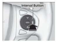
Press the Interval button to change the ACC following-interval.
