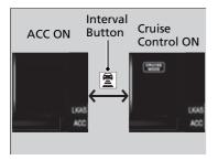
Press and hold the Interval button for one second. **Cruise Mode Selected** appears on the multi-information display for two seconds, and then the mode switches to Cruise. To switch back to ACC, press and hold the Interval button again for one second.
