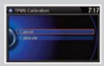
The low tire pressure indicator blinks and calibration begins.
