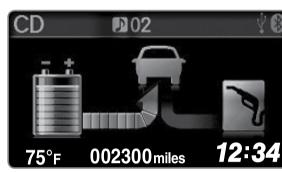
Power is supplied by the electric motor.
