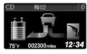
The electric motor is charging the IMA battery.
