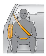
Side airbags are designed to help protect a front occupant's chest and pelvis.
