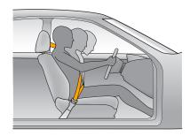
In a moderate-to-severe frontal crash, the seat belts lock to restrain the occupants, and tensioners tighten the front seat belts.
