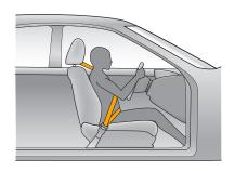
If the driver's seat position sensor detects a driver is closer to the steering wheel than recommended, the airbag will inflate with the least force possible.
