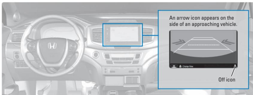
The system does not provide alerts for a vehicle that is moving away from your vehicle, and it may not detect pedestrians, bicycles, or stationary objects.
