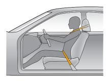
Wearing a seat belt properly and sitting upright helps reduce the chance of serious injuries in all types of collisions. It also helps keep occupants connected to the car and in the best position if the front, side, or side curtain airbags deploy.
