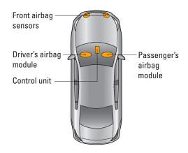
A sophisticated electronic system monitors all airbag systems and the front seat belts whenever the ignition switch is in the ON position. An indicator alerts the driver if a possible problem is detected.
