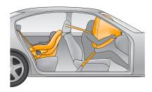
Never install a rear-facing child seat in the front seat. In a severe frontal collision, or if the passenger's front airbag deploys, the child could be killed or seriously injured.
