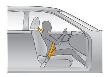
If the driver's seat position sensor detects a driver is closer to the steering wheel than recommended, the airbag will inflate with the least force possible.
