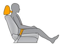
Adjusting a head restraint so the center is level with the back of the occupant's head (or as high as possible for taller people) can help reduce injuries during a rear impact.
