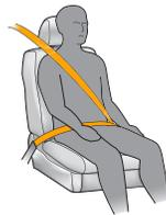
Properly positioned seat belts help restrain occupants and keep them in position in every type of crash.
