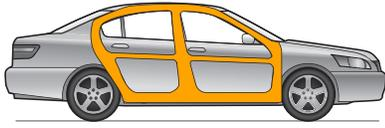
A strong metal frame forms a safety cage around the occupants. Side impact bars across the doors provide additional protection.
