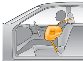
Side airbags can help reduce chest and pelvis injuries to front-seat occupants during severe side impacts.
