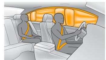
Side curtain airbags can help protect the heads of outboard occupants during a side impact and help reduce the likelihood of ejection in a rollover.
