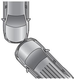
Front airbags are designed to supplement the restraint provided by seat belts in a moderate-to-severe frontal collision with another vehicle.
