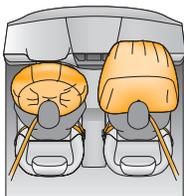
Front airbags supplement seat belts to help protect the head and chest of the driver and front passenger.
