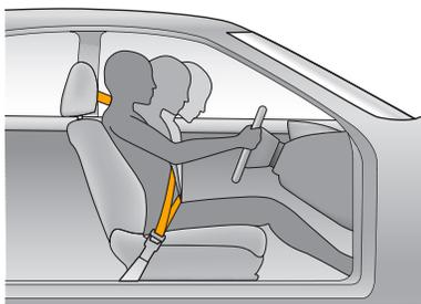
In a moderate-to-severe frontal crash, the seat belts lock to restrain the occupants, and tensioners tighten the front seat belts.
