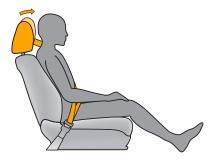
In vehicles equipped with active head restraints, the restraint will move up and forward a little when enough pressure is applied against the seatback.
