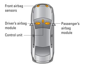
A sophisticated electronic system monitors all airbag systems and the front seat belts whenever the ignition switch is in the ON position. An indicator alerts the driver if a possible problem is detected. If you ever have a frontal crash with another vehicle or a solid object, such as a concrete wall or bridge support, sensors will detect the vehicle's sudden deceleration and send that information to the control unit.
