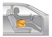
If sensors detect up to about 65 lbs (the weight of an infant or small child) on the front passenger's seat, the airbag will automatically turn off.
