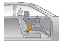
If the driver's seat position sensor detects a driver is closer to the steering wheel than recommended, the airbag will inflate with the least force possible.
