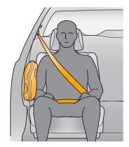
Side airbags are designed to help protect a front occupant's chest and pelvis.
