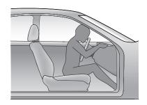
Without a seat belt or an airbag, the occupant will continue forward at 30 mph until they strike the interior of the car with enough force to cause serious injuries.
