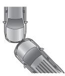
Front airbags are designed to supplement the restraint provided by seat belts in a moderate-to-severe frontal collision with another vehicle.
