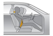
In a moderate-to-severe frontal crash, the seat belts lock to restrain the occupants, and tensioners tighten the front seat belts.
