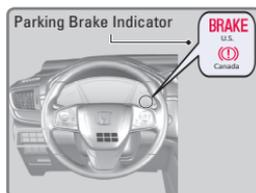
**To release:** Hold the brake pedal down and make sure your seat belt is fastened. Press the switch down to release. The parking brake indicator disappears from the instrument panel.
