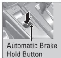
Press the accelerator pedal to cancel brake hold and start moving.
