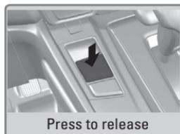
**To release automatically:** Lightly press the accelerator pedal after you have turned the vehicle on, fastened your seat belt, and changed the shift position to either Drive (D) or Reverse (R).
