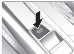
Press the accelerator pedal (or shift into a gear and release the clutch pedal for manual transmission) to cancel brake hold and start moving.
