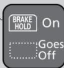
Depress the accelerator pedal while the shift lever is in a position other than P or N . The system is canceled and the vehicle starts to move.
