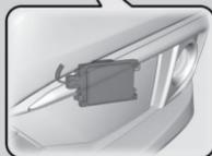
The radar sensor is in the lower bumper. Be careful not to have the radar sensor cover strongly impacted.
