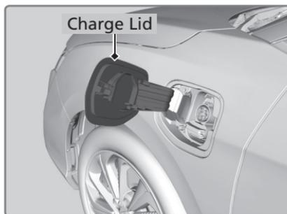
5. To connect the cable to the vehicle, push the cable's charge connector until it clicks to the charge lid. The charge indicator on the charge lid stays on.
