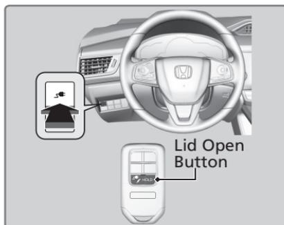
4. Open the charge lid. In case of using with COMBO charge connector, open the charge lid and remove the inlet cover.
