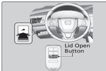
1. The charging cable is stored in a bag in the trunk. Prepare the charging cable and open the vehicle's charge lid. When in use, do not tie or coil the cable.
