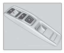
In freezing or sub-freezing conditions, the electronic gear selector response may be slow. Always apply the brake pedal before shifting into Park (P) and confirm that (P) is shown on the gear position indicator before releasing the brake.
