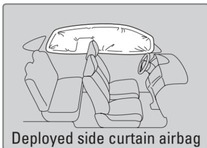
Deployed side curtain airbag
