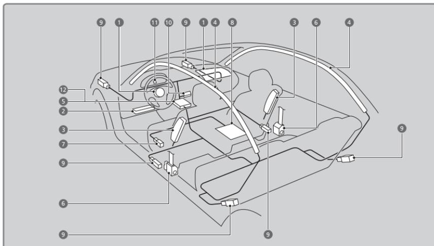
1. Two SRS (Supplemental Restraint System) front airbags. The driver's airbag is stored in the center of the steering wheel; the front passenger's airbag is stored in the dashboard. Both are marked **SRS AIRBAG**.
