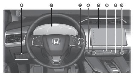
Vehicle Stability Assist (VSA ®) system OFF button Road Departure Mitigation (RDM) button Collision Mitigation Braking System<sup>™</sup> (CMBS<sup>™</sup>) OFF button Charge lid release button
