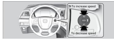
Each time you press the button, the vehicle speed is increased or decreased by about 1 mph (1.6 km/h). If you keep the button pressed, the vehicle speed increases or decreases by 5 mph or 5 km/h until you release it.
