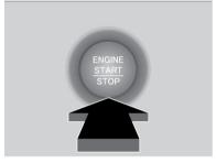
starting the engine. If you press the button and the shift lever is not in Park (P), the vehicle goes into Accessory mode.
