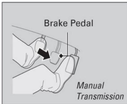
Your vehicle is equipped with disc brakes at all four wheels. The brake assist system increases the stopping force when you depress the brake pedal hard in an emergency situation. The anti-lock brake system (ABS) helps you retain steering control when braking very hard.
