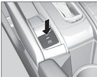
If you pull up and hold the electric parking brake switch while driving, the brakes on all four wheels are applied by the VSA<sup>®</sup> system until the vehicle comes to a stop. The electric parking brake then applies, and the switch should be released.
