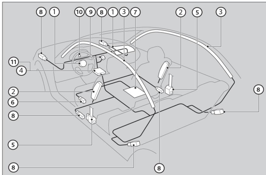
1. Two SRS (Supplemental Restraint System) front airbags. The driver's airbag is stored in the center of the steering wheel; the front passenger's airbag is stored in the dashboard. Both are marked **SRS AIRBAG**.
