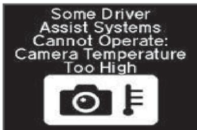
The temperature inside the front sensor camera is too high.
