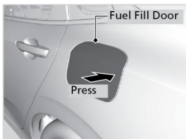
3. Unlock the driver's door using the master door lock switch. The fuel fill door on the outer side of the vehicle will unlock.
