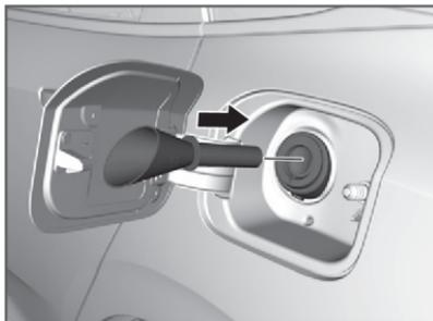
5. Fill the tank with fuel from the portable fuel container. Pour fuel carefully so you do not spill any.
