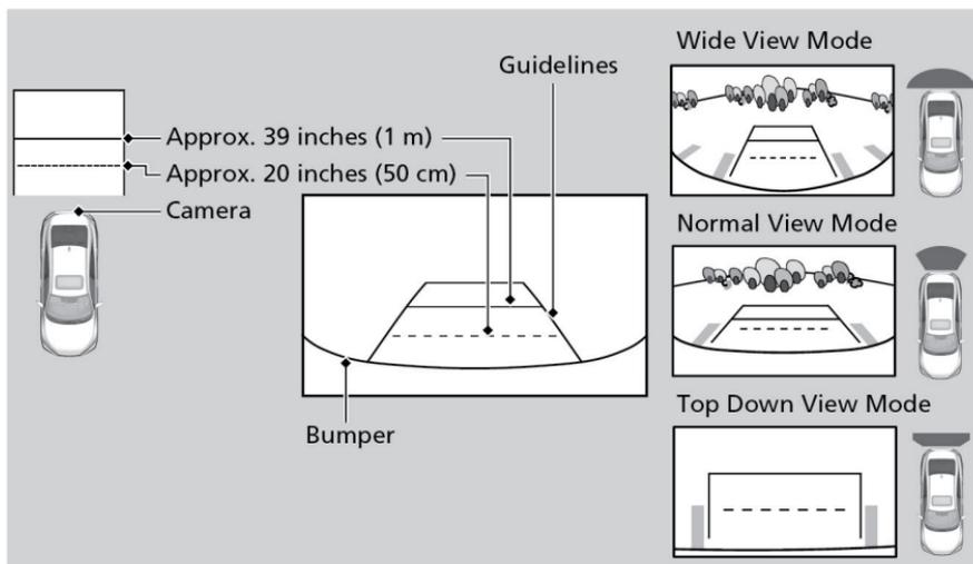
The rear camera view is restricted. You cannot see the corner ends of the bumper or what is underneath the bumper. Its unique lens also makes objects appear closer or farther than they actually are.
