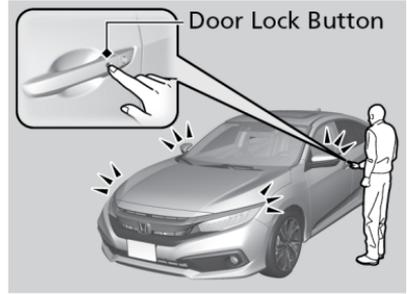
**Note:** System range is affected by radio signals from other devices (for example, cell phones or tablets) so for best results, carry the remote transmitter separately from these devices.
