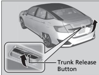
Push up the release button on the trunk lid after the doors are unlocked.
