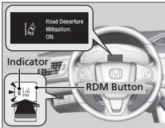
Press the RDM button to turn the system on and off.
