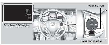
Take your foot off the pedal and press down the **–/SET** button when you reach the desired speed. The moment you release the button, the set speed is fixed, and ACC begins.
