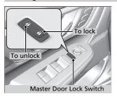
Press the master door lock switch in as shown to lock or unlock all doors and the tailgate.
