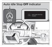
To turn the Auto Idle Stop system off, press this button. The Auto Idle Stop system stops.
