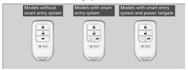
Use the keys to start and stop the engine, and to lock and unlock all the doors and tailgate. You can also use the remote transmitter to lock and unlock all the doors and tailgate.
