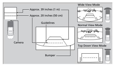
You can view three different camera modes on the rearview display. Touch the appropriate icon to switch the mode.
