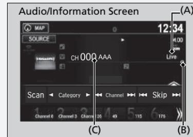
(A): Shows how much time the replayed segment is behind the real-time broadcast
