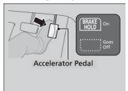
Depress the accelerator pedal while the transmission is in a position other than  $\boxed{\textbf{P}}$  or  $\boxed{\textbf{N}}$ . The system is canceled and the vehicle starts to move.
