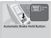
Fasten your seat belt properly, then start the engine. Press the automatic brake hold button.
