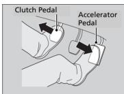
Gently depress the accelerator pedal and release the clutch pedal.
