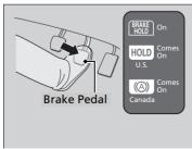
Depress the brake pedal to come to a complete stop.
