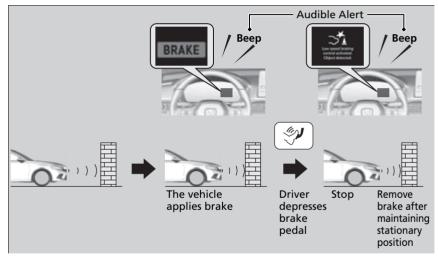
If the only rear sensors are turned off using the parking sensor system, the Low Speed Braking Control is not working when reversing.
