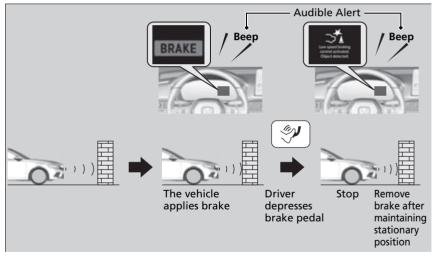
If the only rear sensors are turned off using the parking sensor system, the assistive braking is not working when reversing.
