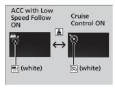
Press and hold the (a) (interval) button for one second. **Cruise Mode Selected** appears on the driver information interface for two seconds, and then the mode switches to Cruise.
