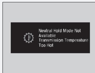
The transmission may not stay in **[N]** position while the following indicator is on:
